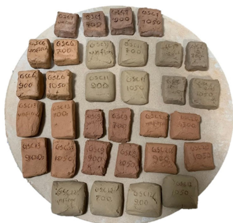
FIGURE 7 Examples of briquettes made for the firing experiment, dimensions of each piece ca. 8 \times 2 \times 5 cm. (Photograph by E. Dammer).
