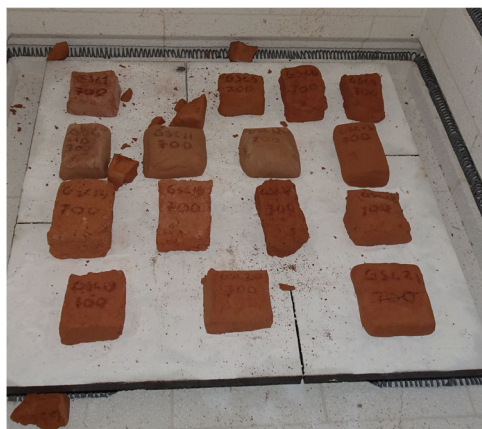
FIGURE 8 State of the sample after the first firing; GSC5 exploded into small pieces. (Photograph by E. Dammer). GSC, Geological Sample China.
